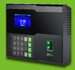
IN05 is a fingerprint identification time & attendance and access control terminal, which can connect with third party electric lock, door sensor and exit button etc.
